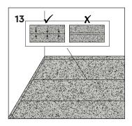
Proceed to cover the entire floor making sure that the joints are butted tight and use an adequate tape to fix it.
