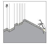
The barrier must also be applied in the perimeter of pipes, ducts or any other component protruding from the floor. Spot adhere the strips to the wall using acrylic glue or a bead of silicone sealant.
