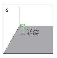
The humidity content of the slab is critical: it must not exceed 2.5 % (MC).
