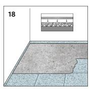
Cast a suitable screed over the loose laid PE foil previously installed over the product.
