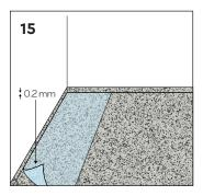
An waterproof membrane (ex. Polyethylene foil) minimum 0.2mm covering the entire flooring area must be installed prior to the screed.
