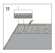
Cut and trim the underscreed to the designed size to fit the installation. Apply directly over the slab. In case of profile material, dimple side must face down.
