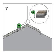
Install a perimeter insulation barrier vertically around the entire perimeter of the room with width equal to that of the floor build up.
