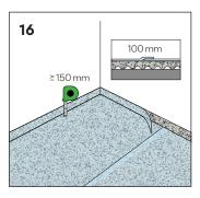
Install it, minimum 150mm wide vertically and overlapping it, minimum 100mm.
