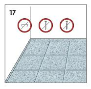
After completion, the insulation vapour barrier should cover the entire underscreed area without gaps. Never mechanically fasten the underscreed or the foil barrier with screws, nails or staples as this will severely diminish the performance of the insulation barrier.
