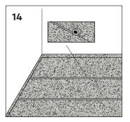
After completion, the underscreed should cover the entire flooring area without gaps and with joints securely taped.
