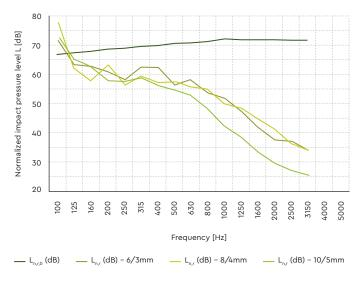
$<sup>{\</sup>bf L}_{\rm ref}$  Normalized impact sound pressure level of the reference floor with the floor covering under test
