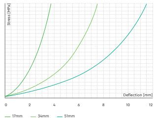
Note: 34mm and 51mm thickness achieved through stacking 17mm (profile) thickness layers. Samples tested –  $300\times300$  [mm]
