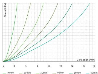
Note: 20mm, 30mm, 40mm, 50mm and 60mm thickness achieved through stacking 10mm (flat) thickness layers. Samples tested – 300×300 [mm]
