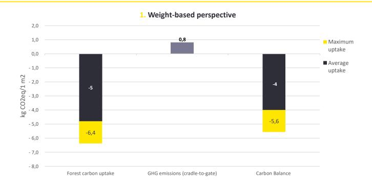
Underlay 5156 VB carbon balance reaches up to:
