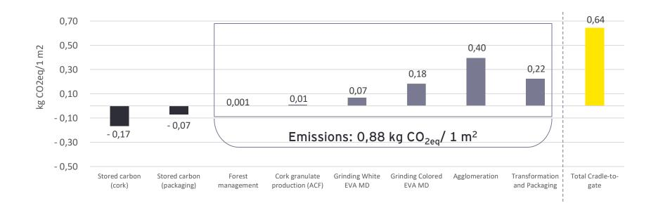
45% emissions associated with agglomeration process, 25% emissions associated with transformation and packaging process and 21% emissions associated with grinding colored EVA process
