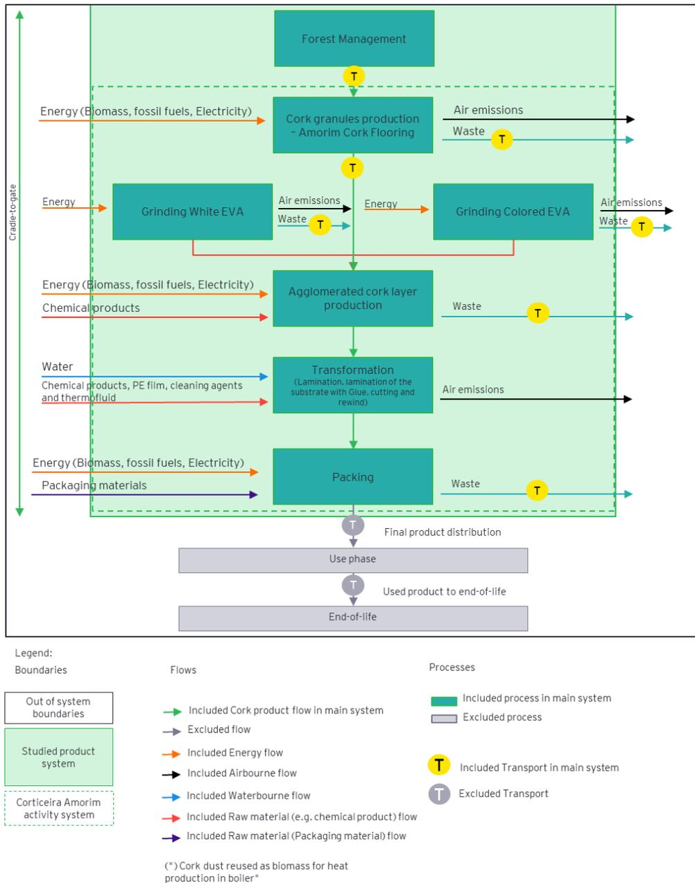
Figure 2 - System boundaries for the Underlay 5156 VB's studied system, relevant flows and processes
