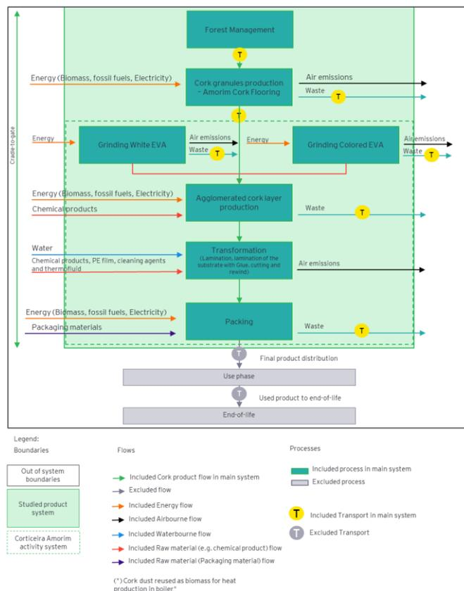
Figure A - System boundaries for the Underlay 5156 VB's studied system, relevant flows and processes
