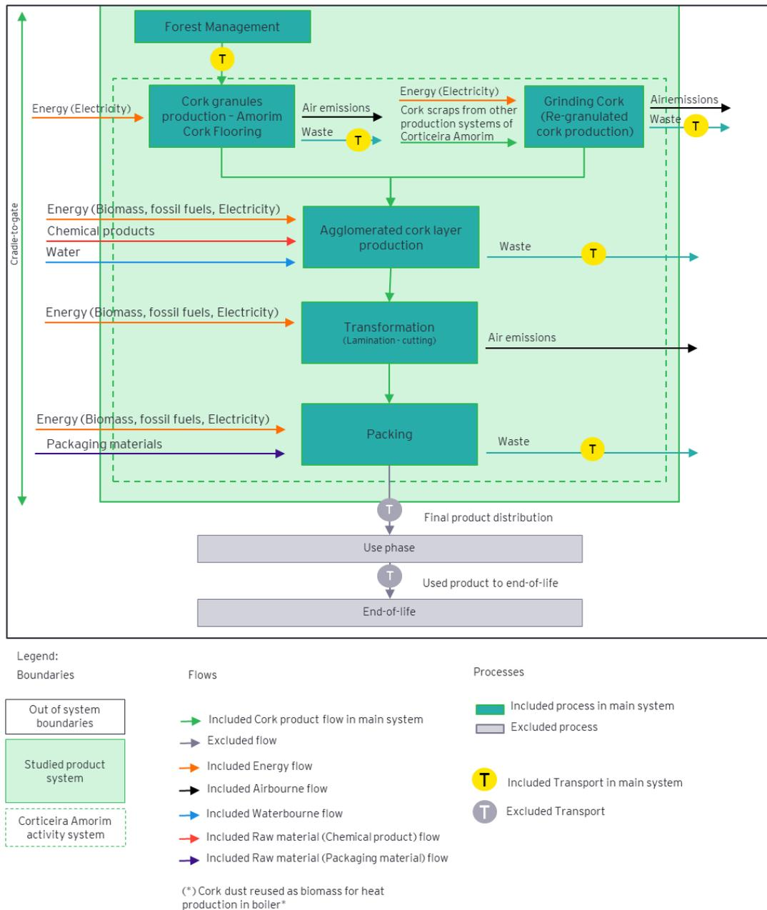
Figure 3 - System boundaries for the Underlay Nature 8210's studied system, relevant flows and processes
