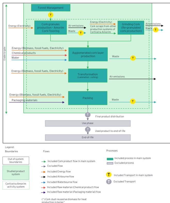
Figure B - System boundaries for the Underlay Nature 8210's studied system, relevant flows and processes
