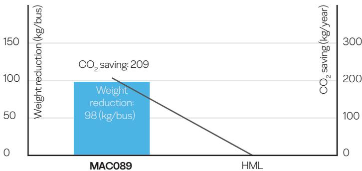
a) comparing against a HML core (2500 kg/m<sup>3</sup>), in a configuration 6/3/6 an 500kg/m<sup>3</sup> plywood
