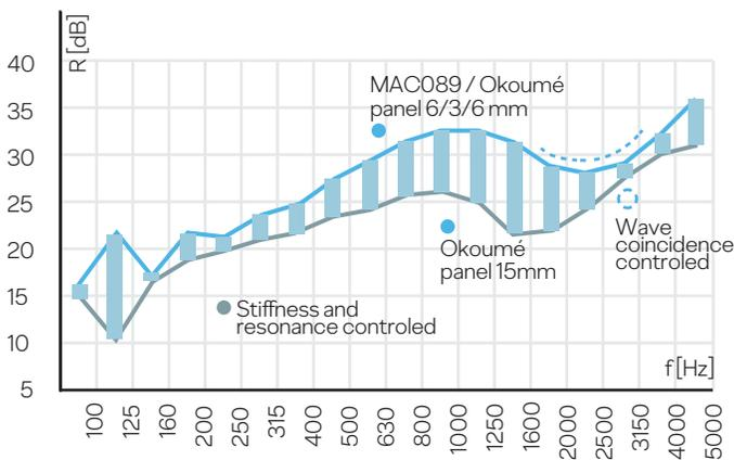
**MAC089** is a multilayer panel material with a very good noise control performance at the mass controlled region and at the medium and high frequency region, while keeping a lower panel weight.
