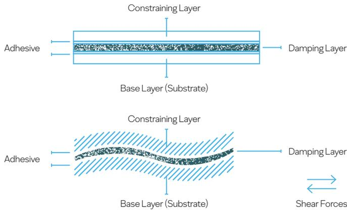
During vibration distortion the system flexes creating shear forces on the constrained layer.
