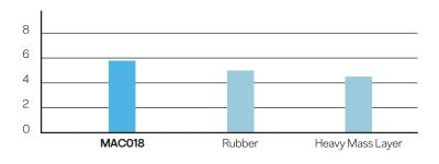
**MAC018** is an engineered cork, rubber and EVA composite material used in multilayer panel constructions as a CLD (constrained layer damper) preventing and dissipating structural vibration before it is transformed into airborne noise.
