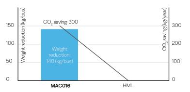
a) comparing against a HML core (2500 kg/m³), in a configuration 6/3/6 an 500kg/m³ plywood
