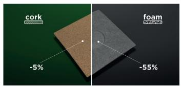
Result: cork proved to be more resilient, with just 5% thickness loss after 100,000 charge cycles.
