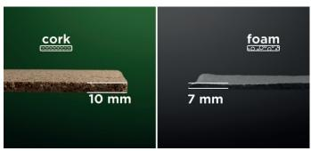
Result: cork delivers superior performance and shows almost the same thickness after being compressed. Less than 10% of thickness loss.
