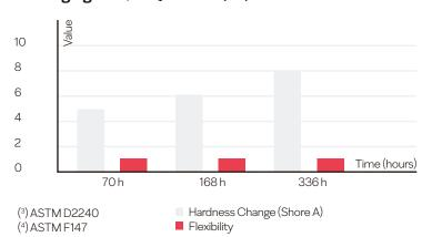
**TD 7000** sealing material is compounded with Silicone (VMQ) rubber. This product is recommended for most transformer oils with an outstanding resistance to extreme temperatures.
