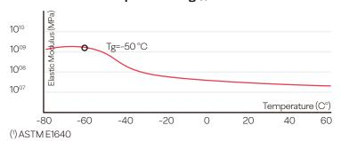
**TD 1310** sealing material is compounded with special Nitrile (NBR) rubber. This product is recommended for most transformer oils with an outstanding resistance to low temperatures.
