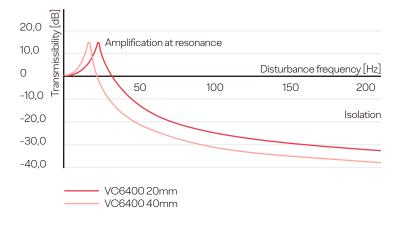
**VC6400** Vibration Control material is a compound engineered with Cork and Synthetic rubber.
