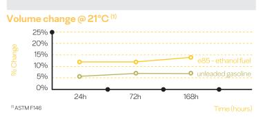
**TS 7110** sealing material is compounded with Epichlorohydrin (ECO) rubber. This product has an outstanding performance for gasoline resistance but it also suited for most engine fluids and application.
