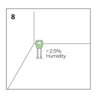
Subfloor preparation: Make sure that the subfloor is leveled, dry, clean and in good structural conditions.
