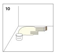
Optinal step: Apply the glue using a trowel. The installation of a moisture barrier is not necessary.
