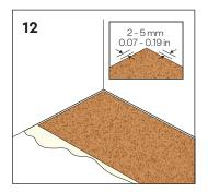
Install the underlayment directly on the adhesive, leave a space between the wall and the underlayment.
