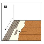
Install the flooring in a perpendicular direction to the underlayment, and let the whole floor dry completely before you start to use it.
