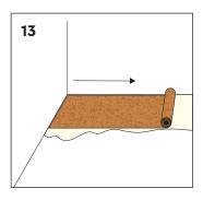
The underlayment should be installed in a perpendicular direction that you plan to install the final floor.
