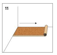
Place one roll parallel to the wall with the vapor barrier face down on the subfloor. The foil overlap should be on the opposite side of the wall.
