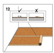
Install the new row immediately next to the previous one, covering the foil overlap. Be sure not to overlap the underlayment edges nor leave any gaps.
