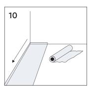
You must first install a moisture barrier across the entire area of the room. It should be installed following the outline of the enclosing wall.
