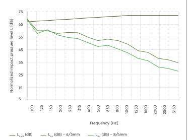
$<sup>{\</sup>bf L}_{{\bf n},{\bf r}}$  Normalized impact sound pressure level of the reference floor with the floor covering under test
