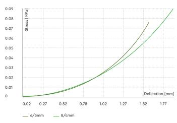
Note: Following ISO8013-1998 measured in Cantilever Test System
