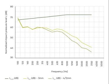
$<sup>{\</sup>bf L}_{{\bf n},{\bf r}}$  Normalized impact sound pressure level of the reference floor with the floor covering under test
