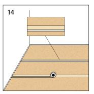
Use a sealing tape to seal the rows securely together.
