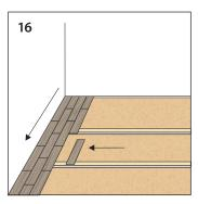
Install the flooring in a perpendicular direction to the underlayment.
