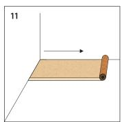
Place one roll parallel to the wall with the vapor barrier face up on the subfloor. The foil overlap should be on the opposite side of the wall.
