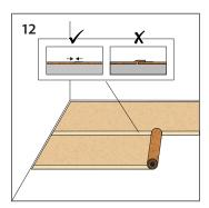
Install the new row immediately next to the previous one, covering the foil overlap. Be sure not to overlap the underlayment edges nor leave any gaps.
