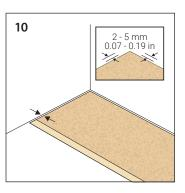
The underlayment should be installed in a perpendicular direction to the final floor. Leave a little space between the wall and the underlayment.
