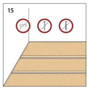
Never mechanically secure the underlayment with screws, nails or staples, since this may undermine its effectiveness.
