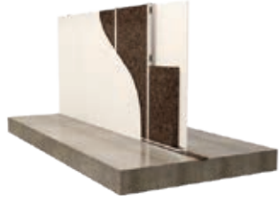
Internal partitions Metal-stud wall and slab discontinuity
