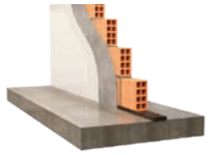
Internal partitions Masonry wall and slab discontinuity
