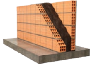
Internal partitions Filling the internal double walls with expanded cork granules
