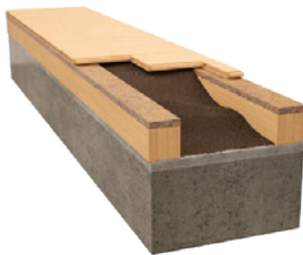
Slab and Floors Resilience on nailed hardwood floor over coconut fiber
