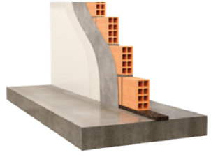
Internal partitions Masonry wall and slab discontinuity
