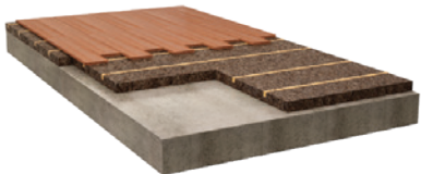
Slab and Floors Lightweight concrete - screed filling
